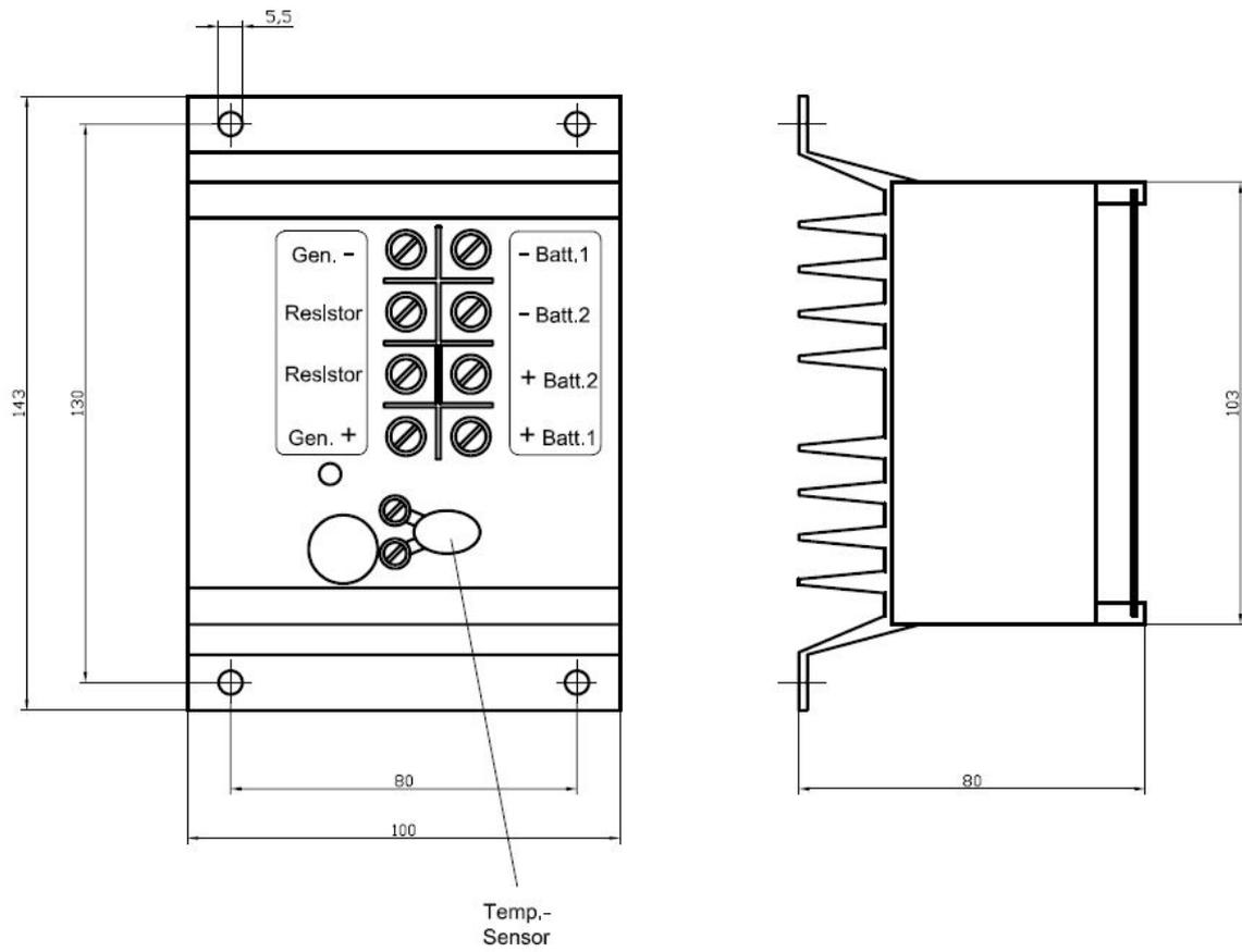
**Dimensions of the power resistor:**
